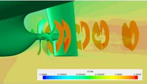
Assess the propulsive efficiency of contra-rotating propellers
